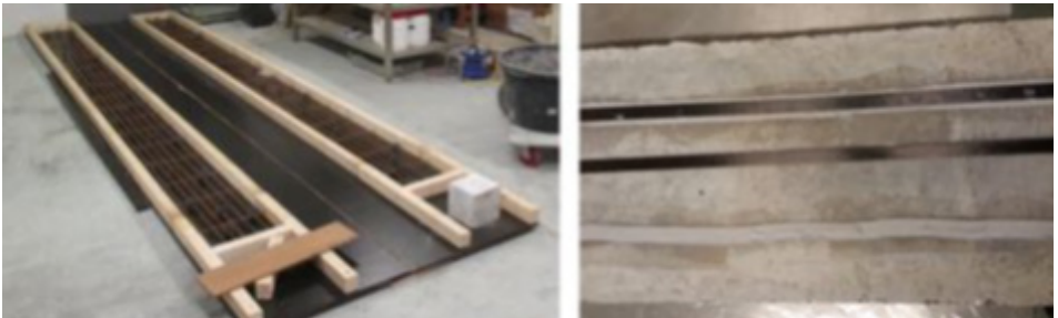
Pictures (a): preparation of the specimens and (b) CTRP bonding
